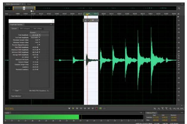
**Figure 15:** Extraction of peak amplitude information from microphone audio recording as point of comparison.
